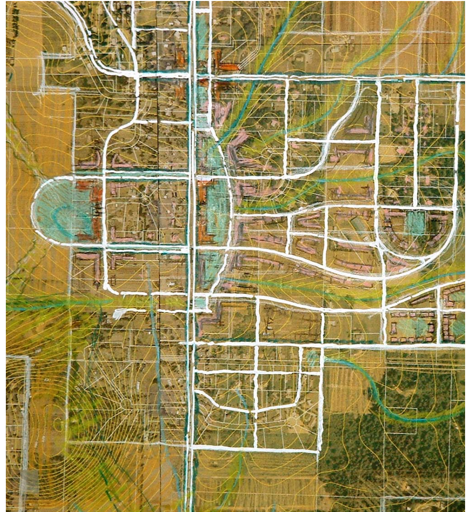
Close up detail from the Green Team rendering showing east central portion of the site centered just south of Wilson's Corner. The attention paid by Green Team members to existing parcel lines, drainage ways, and roads is apparent. The intention was to formulate a plan that could evolve over time through the independent decisions of property owners to develop or add housing to parcels.
