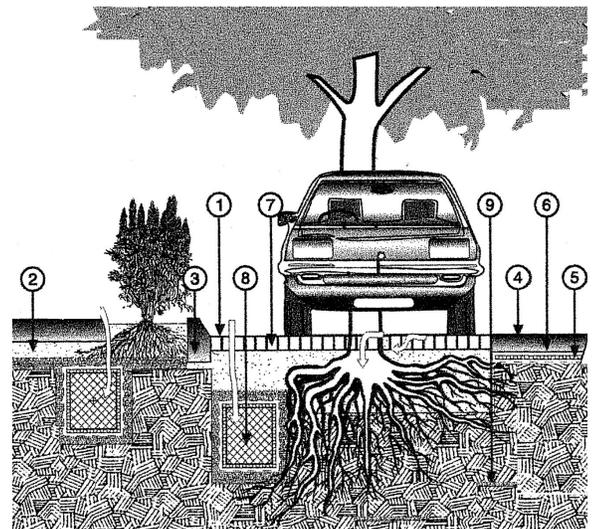
*“The type of system is suitable for retrofitting of existing stormwater drainage systems. The system allows existing infrastructure to be utilized as a surcharge overflow during major storm events, eliminating the major urban floods and allowing water to be recycled naturally or mechanically.”*
