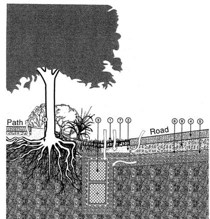
Figure 1-5 - Road drainage system without the curb and gutter:
